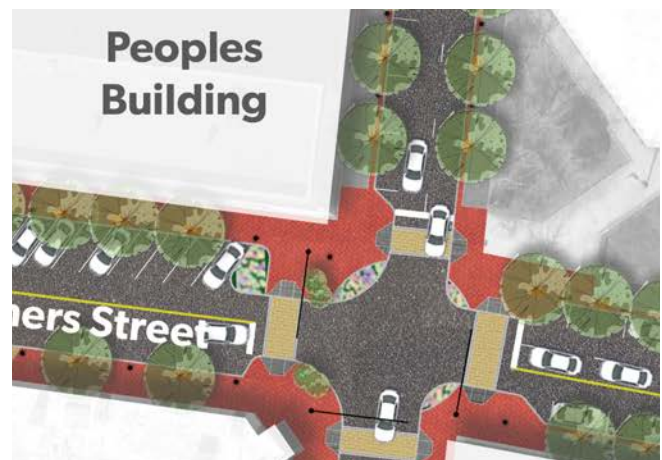
Bump-outs along Summers Street provides sustainable stormwater design compatible with local MS4 codes.
