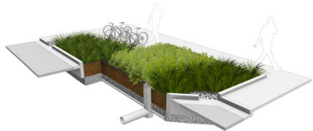
Curb apertures allow for direct stormwater flow into the bump outs.
