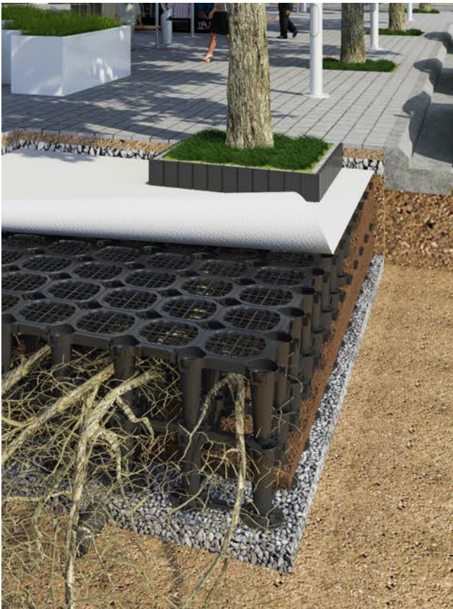
3D Visualization of a structural cell system Source: GreenBlue Urban
